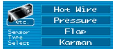
For “Hot Wire”, “Pressure” and “Flap”, press the Right or Down navigation key to go to the sensor number selection window.
