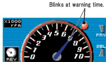
When you want to change an indication item to another, press the Down navigation key(SEL). Now, only the icon remains bright. Use the Up and Down keys to move the cursor over the channel you want to change. Change the indication item that you want to change with the Left and Right keys. After the change is finished, press the Down navigation key(SEL) to go back to the usual monitor display.
