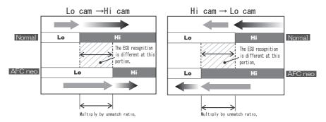
When VTEC changeover point has been changed in the AFC neo, improper fuel injection is performed because the ECU does not recognize the actual cam status. This correction is performed so that the fuel adjustment may not be shifted at that time.
