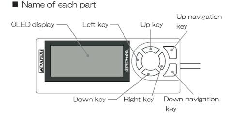
When the left/right-side installation function is set to  $\rm \H{L}eft$  , the names are assigned as follows.
