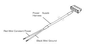
\* It is also possible to connect the Power Supply Wiring Harness directly to the Battery.
