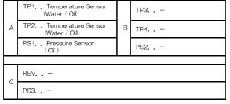
In the case of using 409-A003 Meter, then, the [B] and [C] couplers will not be used. Even if connected the [B] and [C] couplers, the contents will not be displayed.
